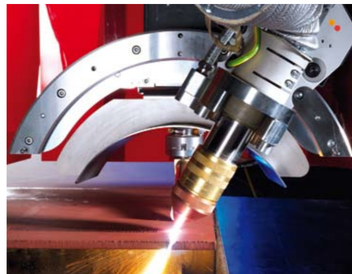
11 | Bevel cut in an angle range of +/- 45° to a material thickness of 30 mm on all geometries
