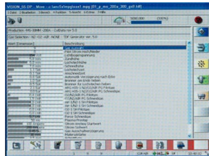
5 | Automatic settings of process parameters for the machine and plasma via TDF files
