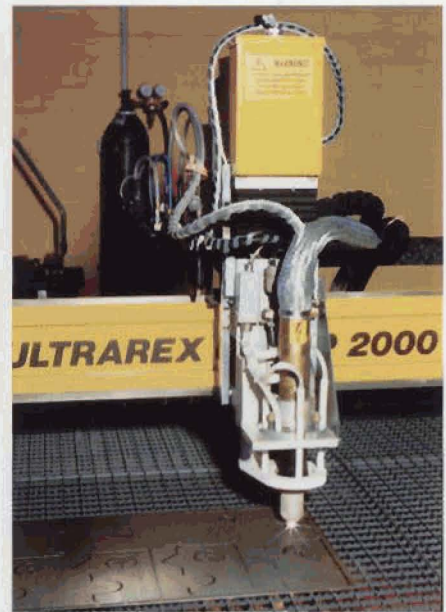
Dynamic plasma cutting process
