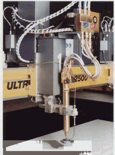
Single-torch unit with a MultJet torch and internal ignition
