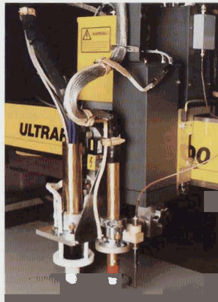
Combined plasma marking and cutting tool for optimized working process
