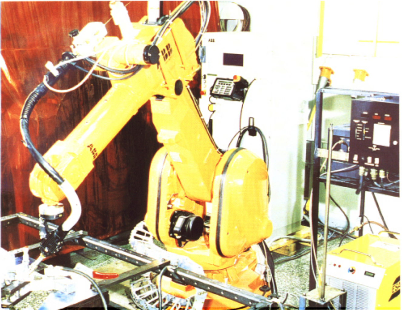
The welding cell used to join extrusions for an all-aluminium passenger car engine cradle. The cell contains an ABB IRB2400 robot, an ESAB Digipulse 450i power source, and a Binzel WH455 welding torch.
